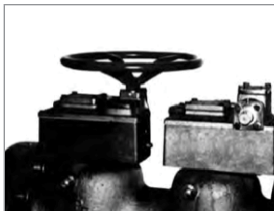
The gear has fixed stops at extreme position, plus position indicator
