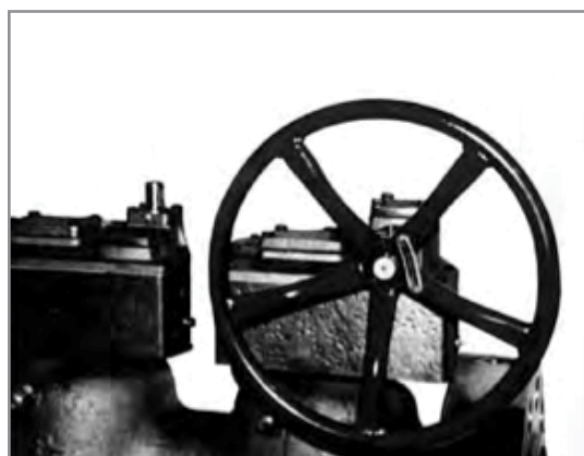
The gear has fixed stops at extreme position, plus position indicator
